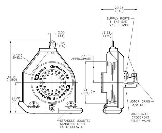
Specifications are based on hydraulic flow of 60 GPM at 2000 PSI
